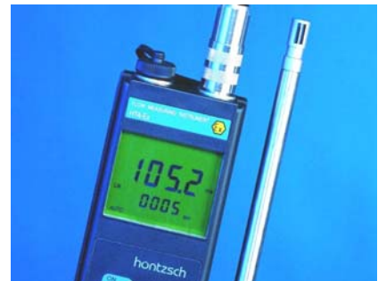
Sensor TA10 ... ZG1b (left) for use with transducer U10a (above right) and hand-held HTA and HTA-Ex (below right)
